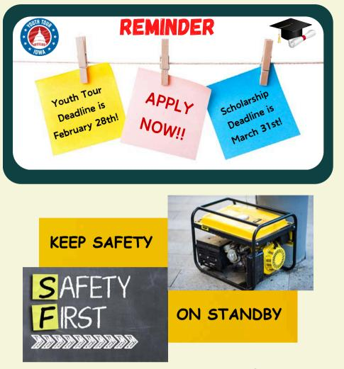
A standby emergency generator is useful during a power outage... if properly installed and used safely. Installation should be done by a licensed electrician to avoid voltage feedback. If a generator is connected to a home's wiring without a transfer switch, power can backfeed along power lines and electrocute utility lineworkers.
